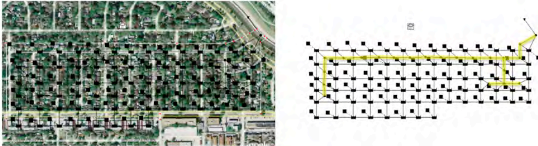
Figure 24: Lazybrook Analog layout. Left panel is SWMM model overlay on aerial image of watershed. Right panel is link-node array without background. Yellow shading indicates subsurface sewer system(s); Blue shading (none in this model) indicates drainage channels.
