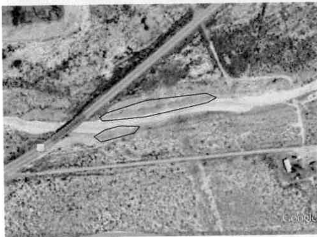
FIGURE 10 Image from 2005 (note bed material piled along stream upstream of bridge location, indicated by closed shapes).
