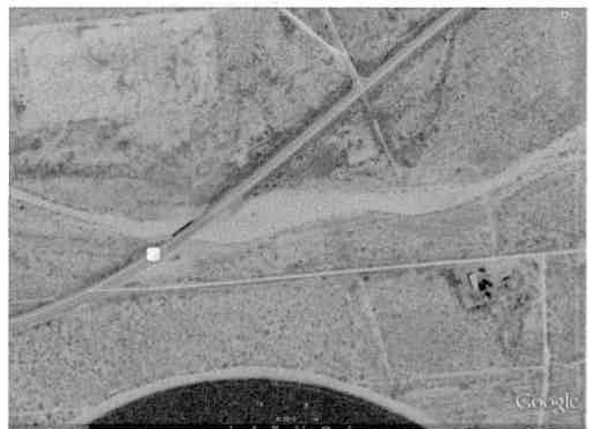
FIGURE 2 Current overhead image (note overwidened section upstream of bridge and appearance of shorter meander wavelength).
