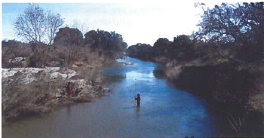
Fig. 2. (Color) USGS personnel surveying on December 15, 2004, one of four stream cross sections to support a slope-area computation of peak discharge for a historically important event at USGS streamflow-gauging station 08148500 North Llano River near Junction, Texas (Photograph by W. H. Asquith and courtesy of USGS)
