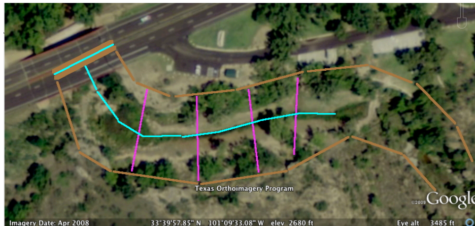
Figure 2. Aerial view of White River case study. The annotated segments indicate approximate location of thalweg, dam, and surveyed cross sections. Additional elevation locations are not depicted on the figure. Flow is from left to right in this photograph. Base image from Google Earth (2011).
