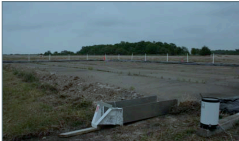
Figure 2: Photograph looking upstream from the outlet for the concrete surface watershed. Diagonal dimension from H-flume to orange cone in far corner is \approx 111 feet. Dimensionless slope along the diagonal is 0.0025
