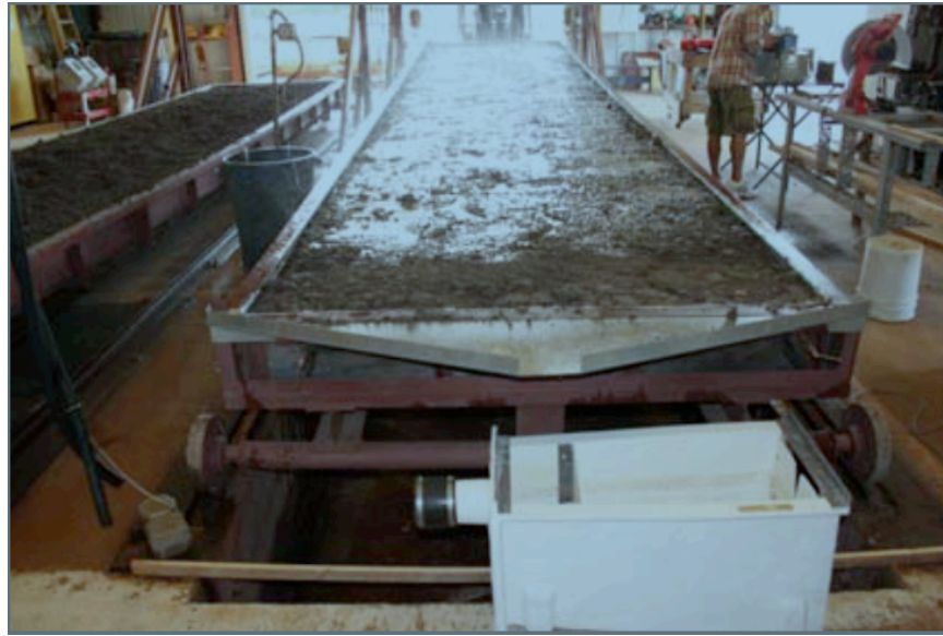
Figure 4: Photograph looking upstream from the outlet for the rainfall-simulator watershed. Longitudinal dimension from the outlet (foreground) to the end of the watershed is 30 ft.
