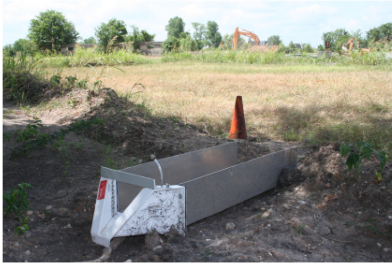
Figure 3: Photograph looking upstream from the outlet for the concrete surface watershed. Diagonal dimension from H-flume to the far corner (left of the orange machinery in the image background) is \approx 111 feet. Dimensionless slope along the diagonal is 0.0025
