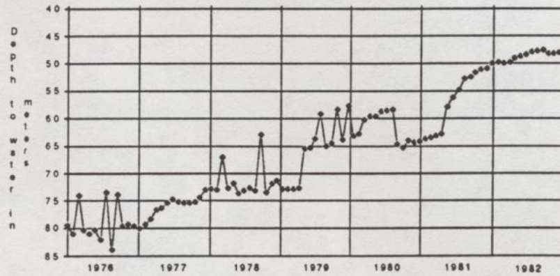
Figure 2 Water level changes: Baytown area well LJ-65-16-930, 131 m depth (1976-1982).
